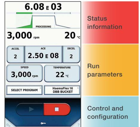
Easily set current parameters and monitor centrifuge status
