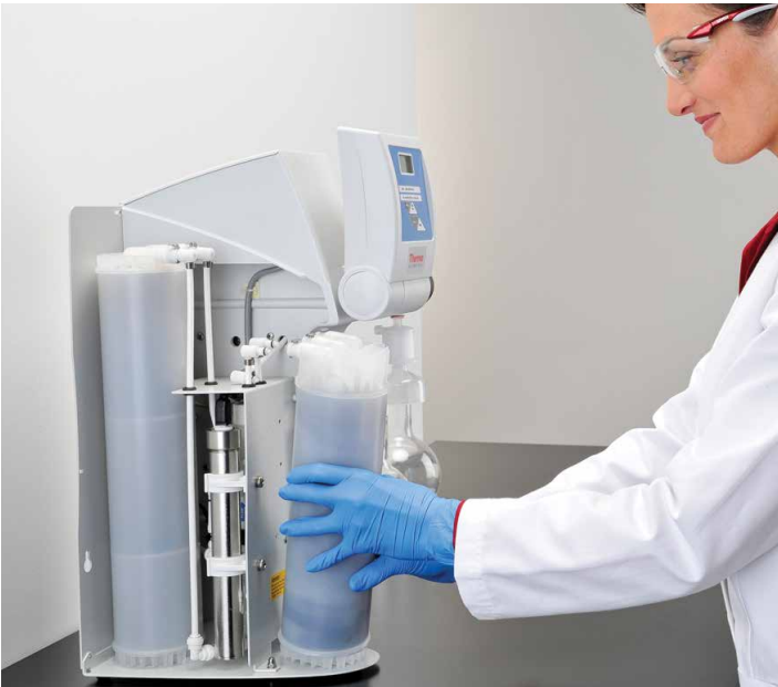
Economical design. The RO membrane cartridge is separate from the DI cartridge, ensuring you only replace each cartridge as needed.
