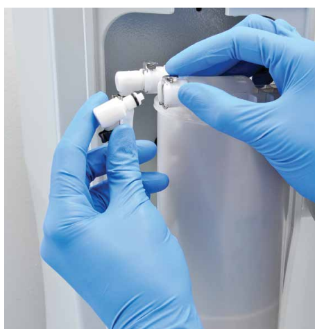
Rapid cartridge change with Aquastop quick-connect design
