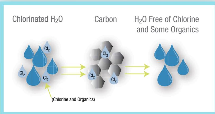
Feed water with organic and chlorine contaminants come into contact with the activated carbon in the cartridge. The impurities adhere to the surface of the carbon, purifying water.
