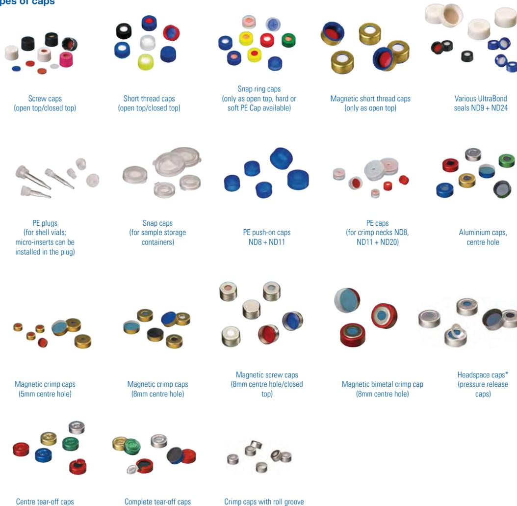
\*A headspace cap is a safety cap for headspace analysis, which should avoid explosion of the vial in case of too much internal pressure. The headspace cap has special score-lines with bridges that break open at an inner pressure of  $3.0 \pm 0.5$  bar. Thus the excess pressure escapes and the risk of vial explosion is avoided.
