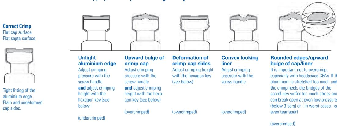
Note that a poor crimp cannot be recognised by simply trying to turn the seal, because PTFE-laminated liners have a very slippery surface, which permits even correctly crimped caps to be rotated if sufficient force is used. Correctly crimped caps can also be turned easily when the liner is in contact with the reduced surface area of a headspace (bevelled top) glass rim.
