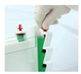
Continue to tighten the screw-pins until the gel clamps glide out of the resting slots and fix firmly against the glass plates pushing them upright.
