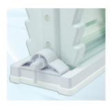
Check the bottom of the glass plates to ensure that they are flush together, and place the PAGE insert on the casting base; make sure that the cams are facing downwards.
