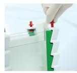
Insert a gel cassette into each side of the inner buffer chamber in the PAGE insert, and begin tightening the vertical screwnins
