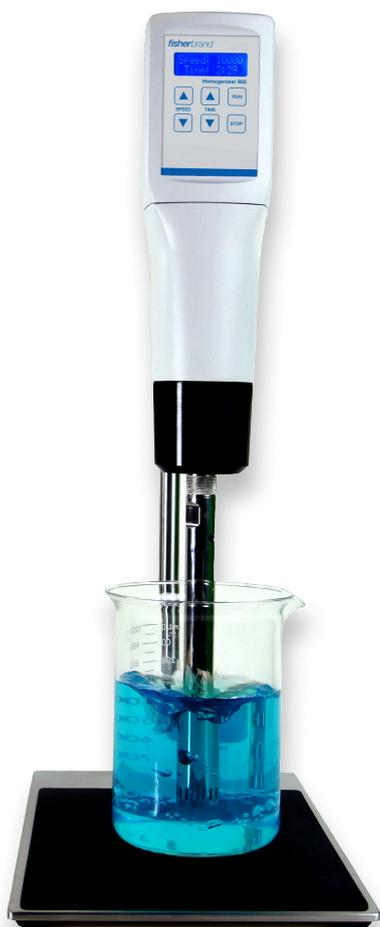
The Homogeniser 850 is an affordable, high performance instrument capable of processing virtually any laboratory sample in seconds. A powerful 850 watt motor provides maximum versatility for homogenising, dispersing or emulsifying the largest variety of sample types and sizes in its class.
