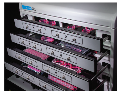
BioSpa processes up to 8 microplates or other labware at a time.
