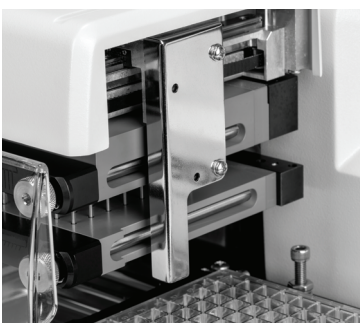
The Verify module is built-in above the manifold and determines the fluid volumes in each well following dispense and aspirate cycles.
