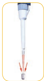
Press FLOWMI onto pipette tip
