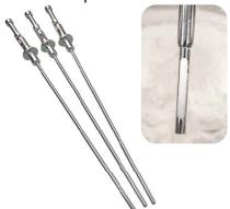
The Powder Sampler Mini is a stainless steel sampler for small quantities. When the button is pressed, a sampling rod enters the sample material and retracts again when released. Thus, a fixed amount of sample material is enclosed in the sample notch of the rod and removed. The sampler precisely collects 0.01 ml, 0.05 ml and 0.1 ml sample volumes, depending on the version. With an insertion depth of up to 300 mm, multiple target point samples can be
